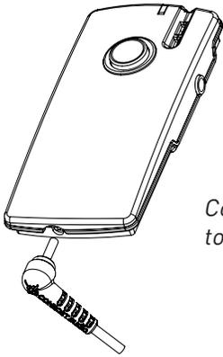
Connecting a charger to the Microphone DM10
