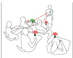
Figure 3: The student microphones shine red to indicate that someone else is using the channel.
