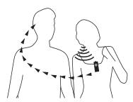
The Microphone DM10 is a microphone for closer range. It works best if worn approx. 12 inches (30 cm) from the mouth.
